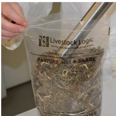
You will need to continue this process on enough bales so that you fill the bag to the specified height. If in doubt, more sample volume is better than less. Usually 10-20 cores will fill the bag.
