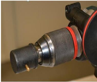
The end piece can remain on the drill while you empty the core sample into the bag, then simply re-attach tube to end piece and core another sample
