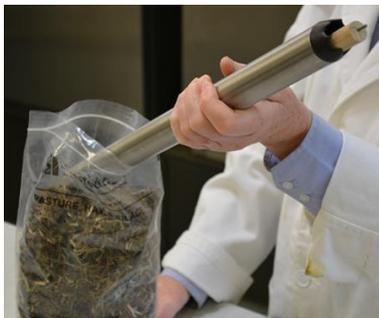
Once you have removed the coring tube from the end piece, empty the contents of the tube into the bag. Use the dow to push the sample through the tube from the cutting end as shown in the photo.
