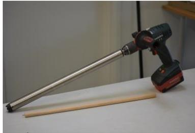
You will get a hay corer and a piece of dowel with a nail in the end.
