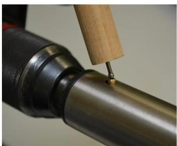
Use the nail to push the gold locking pin in, and twist tube to remove from end piece.
